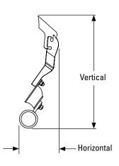
**Horizontal Clearance Required** 7" (175 mm)
